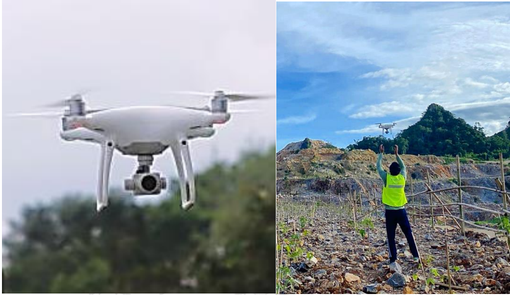
Figure 9 Phantom 4 Pro V2.0 UAV (left), landing after finishing mission by manual catching (right), due to unstable ground surface.
