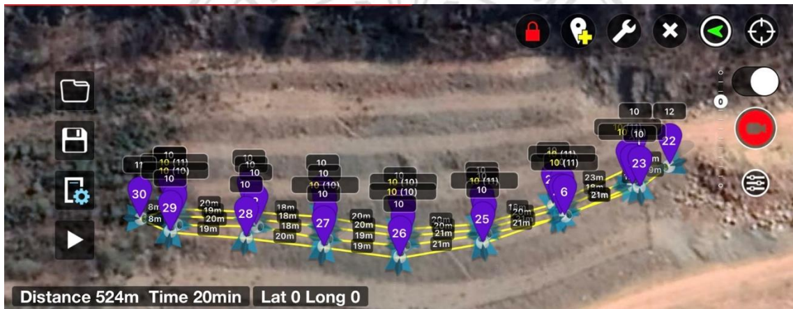
Figure 10 UAV waypoint mission in Litchi flight planner, for 1 st bench; indicating the above ground height of each waypoint; 4 route lines with different camera angles.
