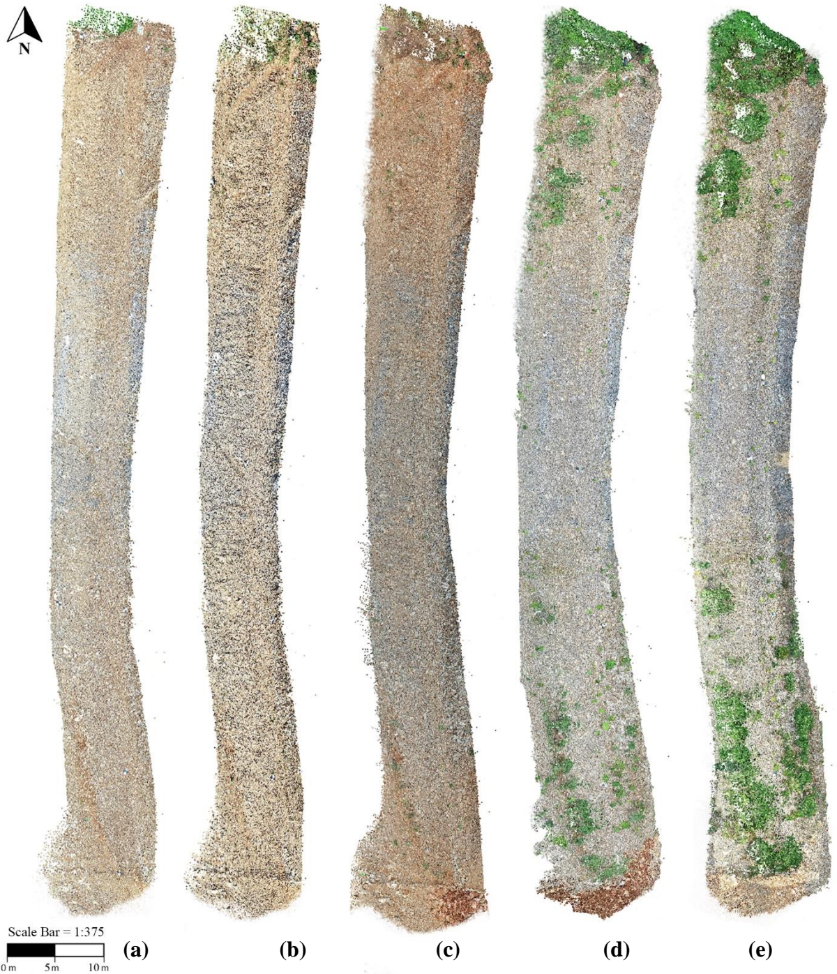
Figure 37 The 3D point clouds of 3 rd Bench. In the order of the first data collection to last data collection (left to right); a-e , respectively. The letter “N” to represent North
