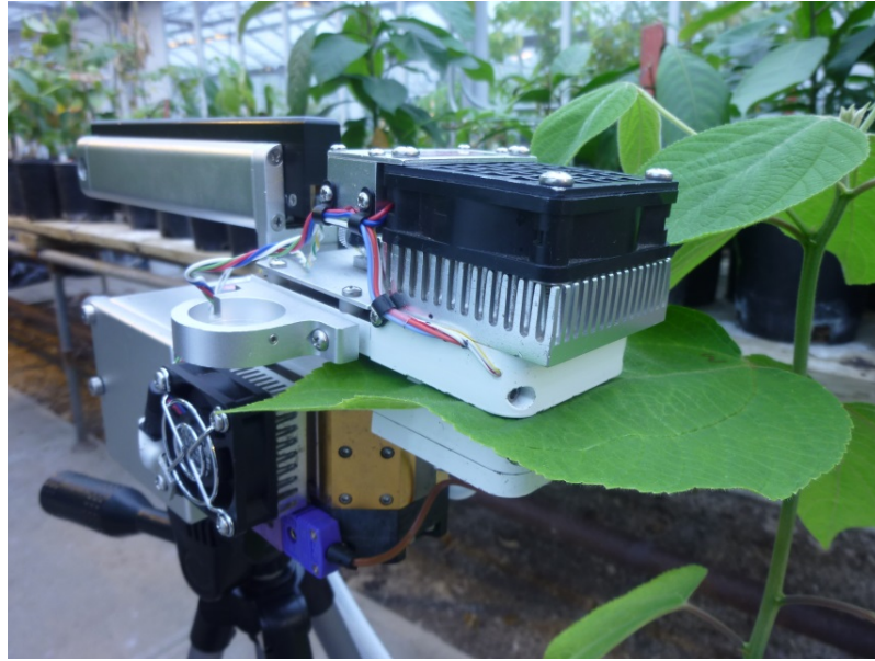
Figure 3.17 Set-up for photosynthesis measurements using the LI-6400
