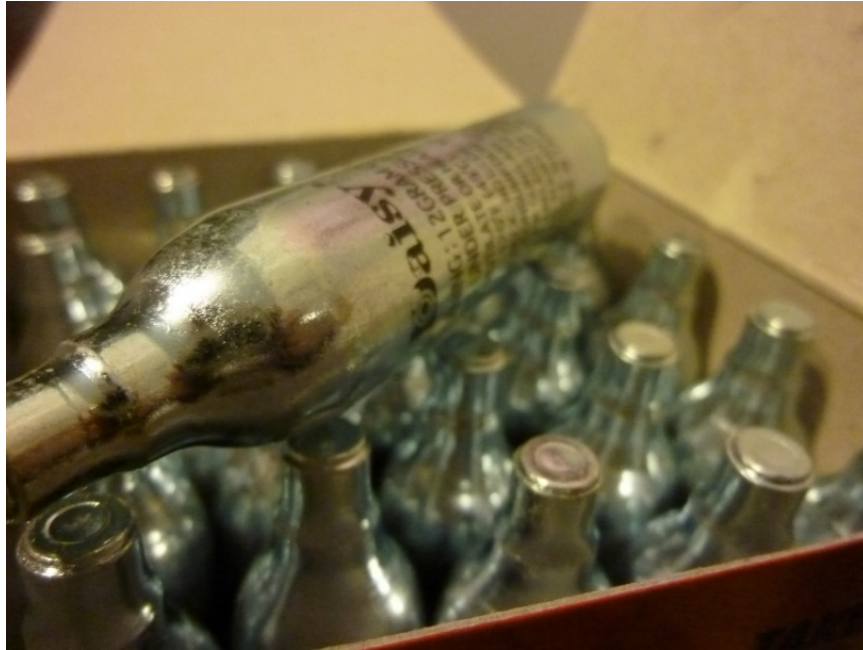
Figure 2.10 CO 2 cartridge used as the source of CO 2 injected.
