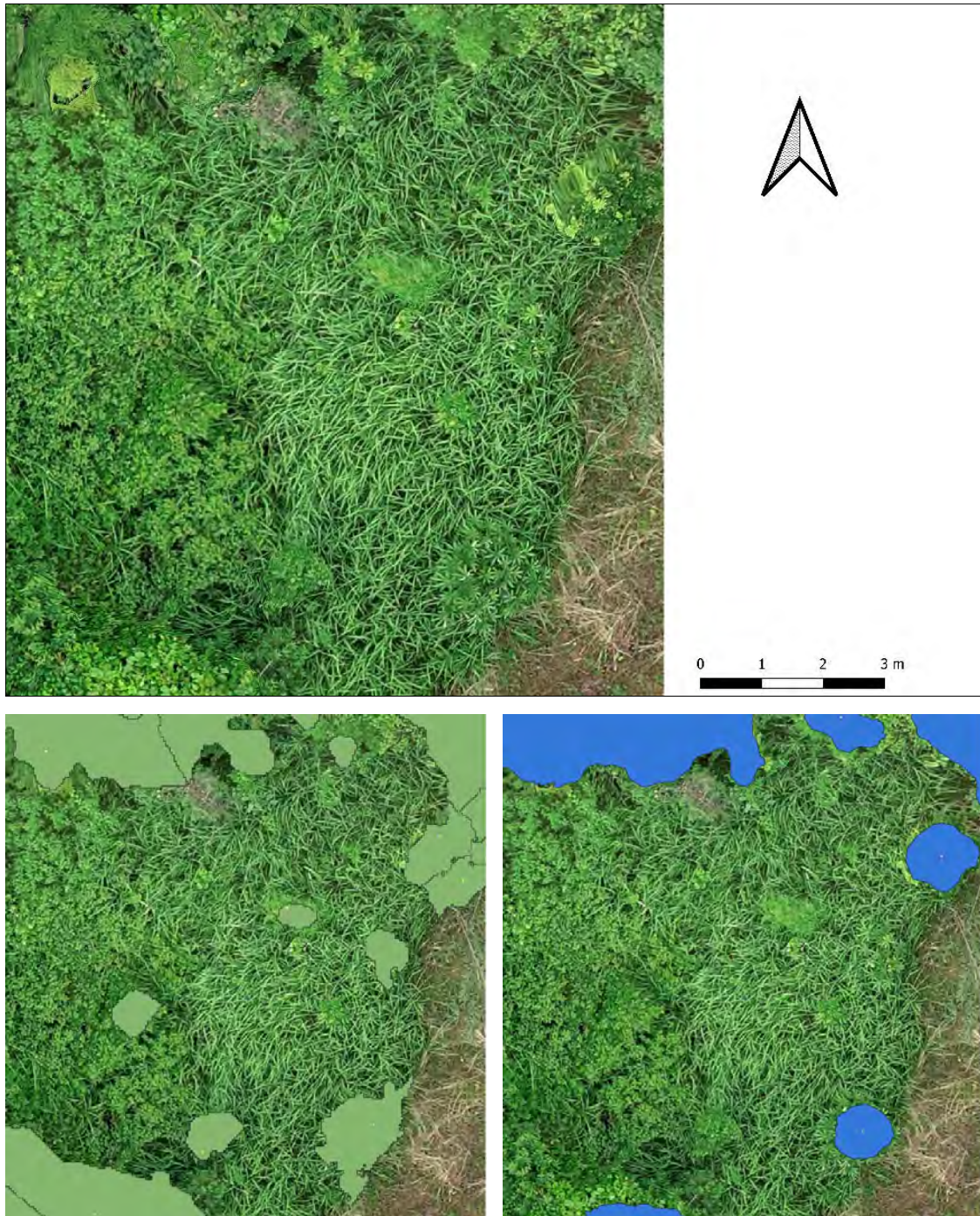
Figure 5: (top) Orthophoto for reference; human eyes can hardly find the small trees emerging above the weed cover (Left) Algorithm-based R package (ForestTools); several trees are detected. (Right) Deep learning-based platform (Picterra); only two trees are detected.
