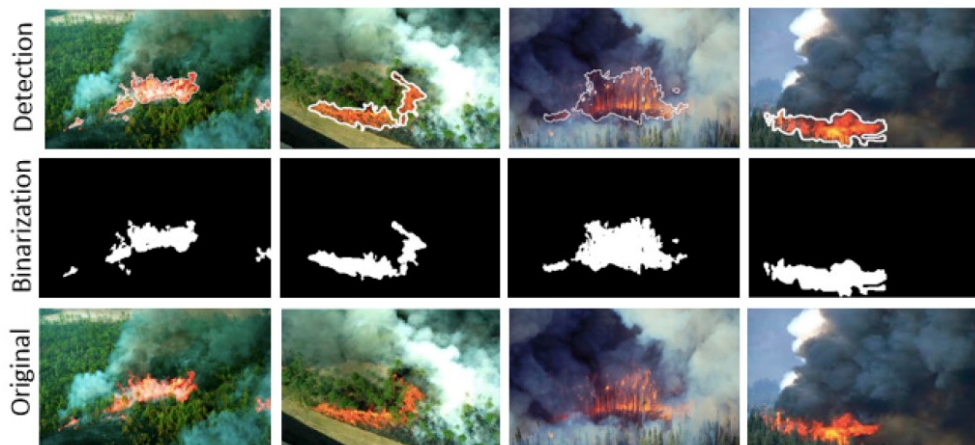
Figure 2.2 – Forest fire detections from UAVs (modified from Cruz et al., 2016)
