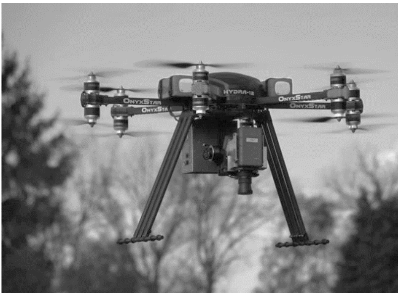
Figure 2.4 - A UAV, equipped with hyper-spectral camera for research in Belgium (CARGYRAK, 2016)
