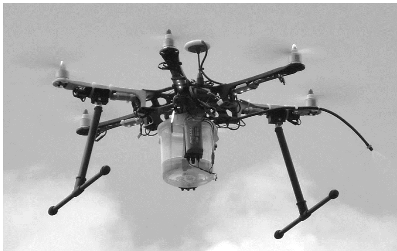
Figure 2.6 - A multi-rotor UAV, equipped with a liquid-storage and spraying system (Photo by Stephen Elliott)
