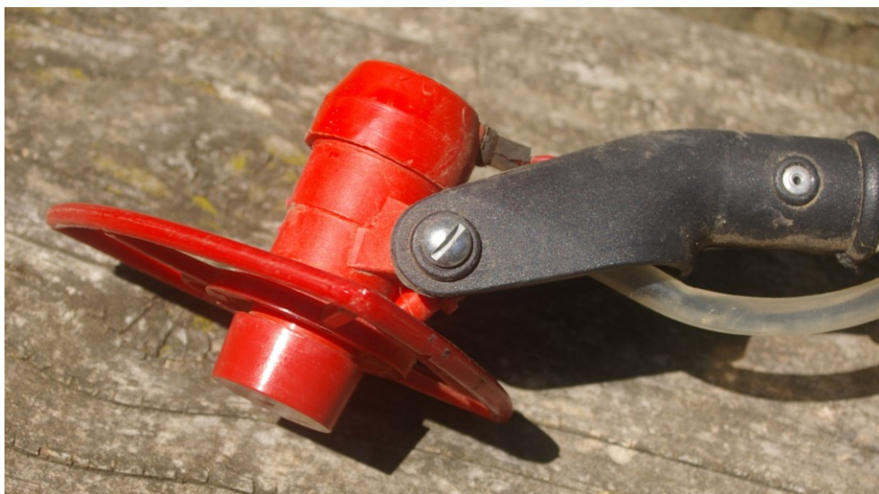
Figure 9.7 - Controlled droplet (spinning disc) nozzles could potentially be used to apply herbicide from on drones. They use low volumes and create large droplets, which would reduce non-target damage.
