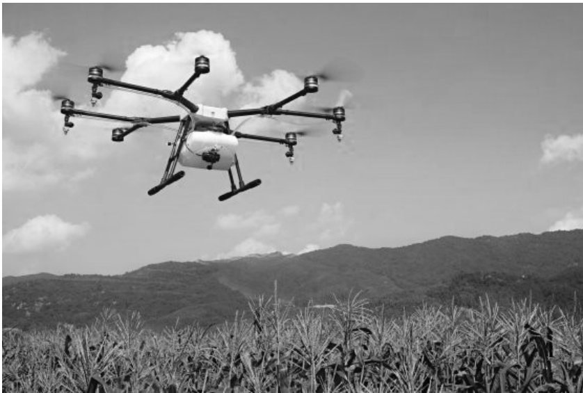
Figure 9.4 – DJI’s Agras MG-1S is an eight-rotor craft spanning 1.47 m with a 10-litre liquid capacity. It is priced at US$15,000 (Photo: DJI)
