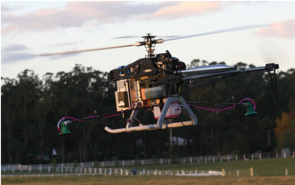
Figure 9.6 – An auto-piloted mini helicopter, used for weed control
