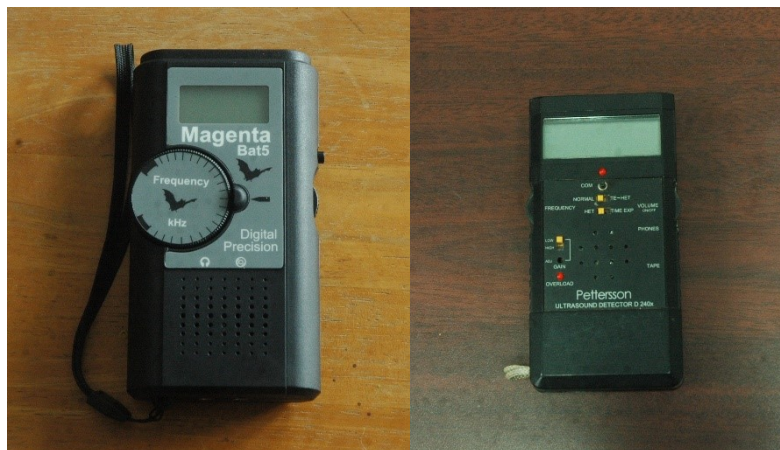
Figure 14.4. A heterodyne bat detector (left) and a time expansion bat detector (right) (Photo: Sara Bumrungsri)
