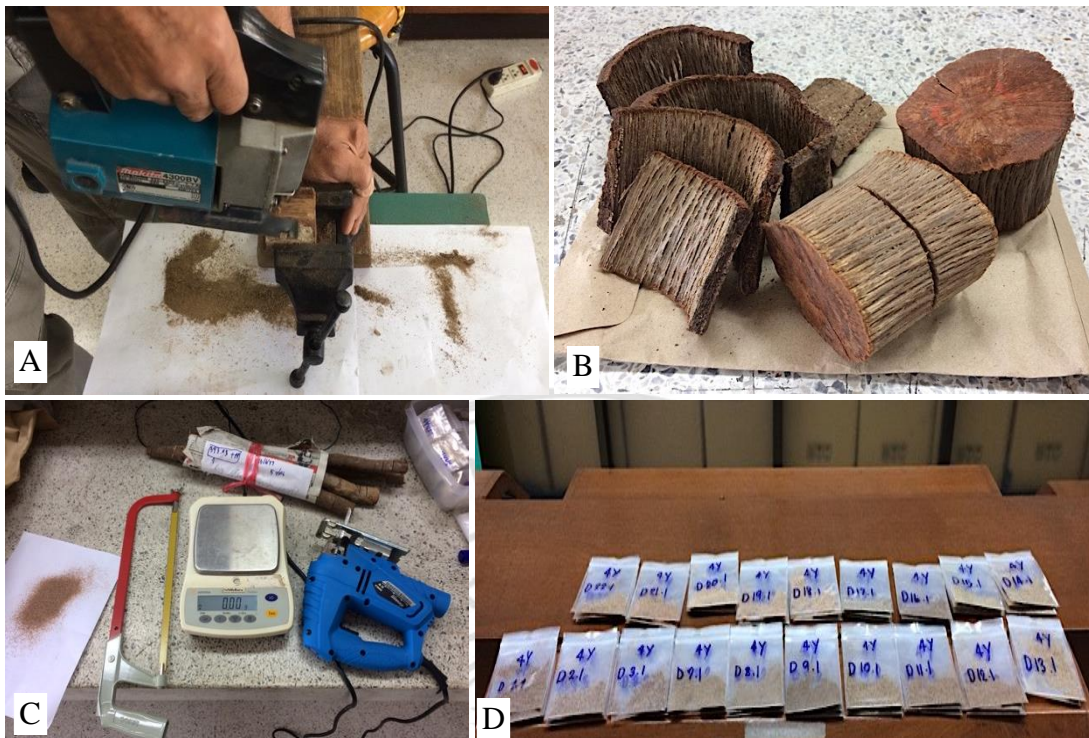
Figure 3.24 Grinding disc and branch samples. (A) Grinding disc samples using a power jigsaw. (B) Ground disc samples. (C) Grinding branch samples. (D) 150 mg ground disc samples in each zip lock bag.
