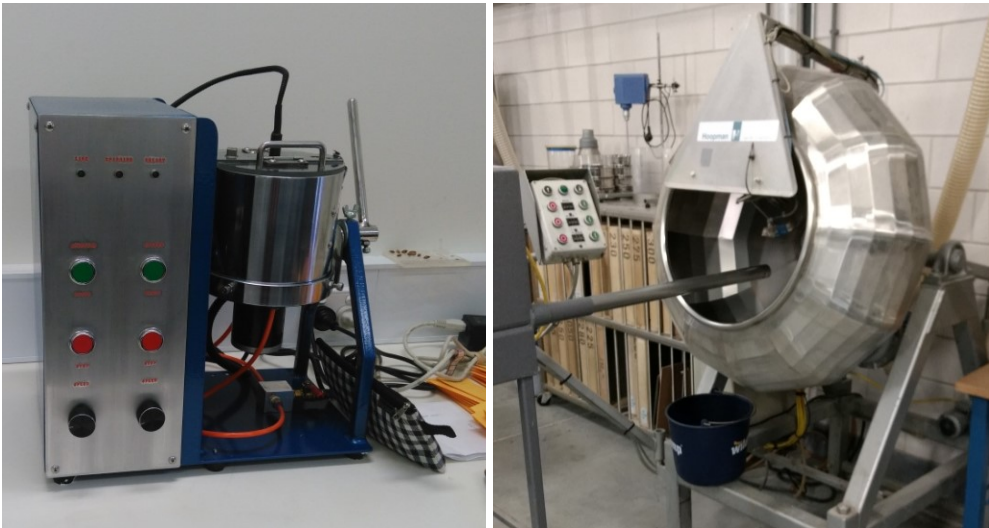
Figure 9.3 – Seed-coating equipment, lab-scale rotary coater on the left, rotating pan on the right.
