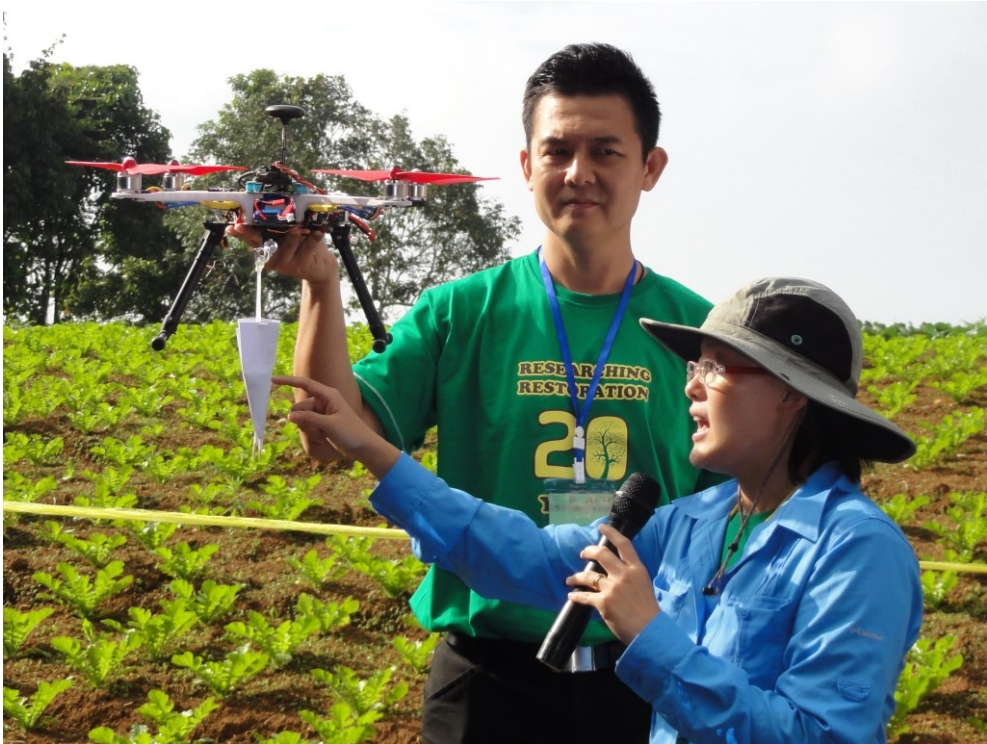
Figure 1.1 - During the workshop field day, prototypes of various technologies that might assist forest restoration tasks were demonstrated. Here a drone, developed by CMU Physics Department, prepares to drop tree seeds in simple paper seed bombs, containing seeds, forest soil and hydrogel.
