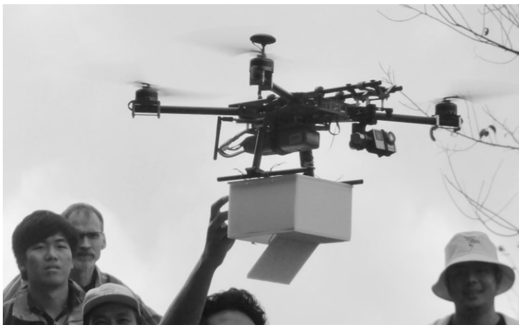
Figure 1.3 – This drone, demonstrated during the workshop field day, uses a simple box with a trap-door to release seeds into deforested sites.
