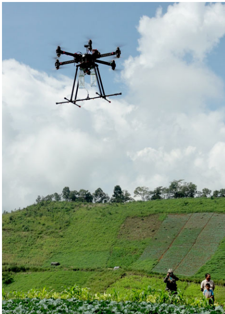
FIGURE 1. Drones, capable of spraying herbicides (and other liquid pesticides), whilst remaining stable, are already being used in agriculture. This one, which carries 2 Litres, was developed by Bird's Eye View (BEV), Chiang Mai. For AFR, such spraying ability must be matched with AI to direct herbicides onto weeds, without spraying tree seedlings and saplings.
