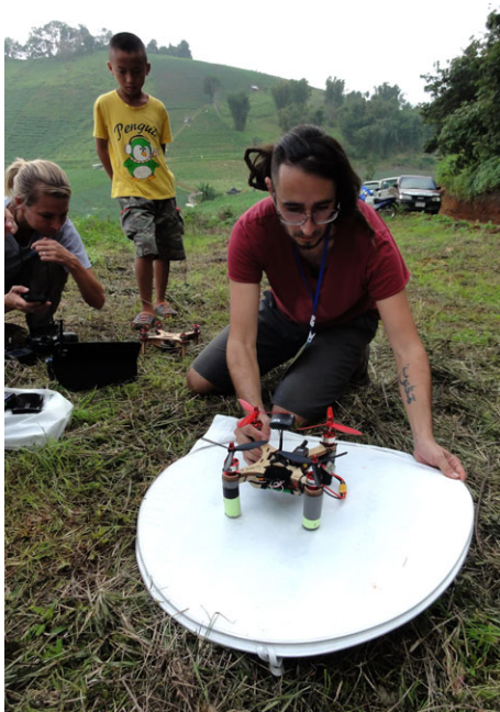
FIGURE 3. Flones are low-cost, self-assembled drone kits, with biodegradable wooden frames, controlled by free, open-source, smart phone apps. They are perhaps the easiest way to involve local communities in simple forest restoration tasks, such as monitoring progress with digital photography.
