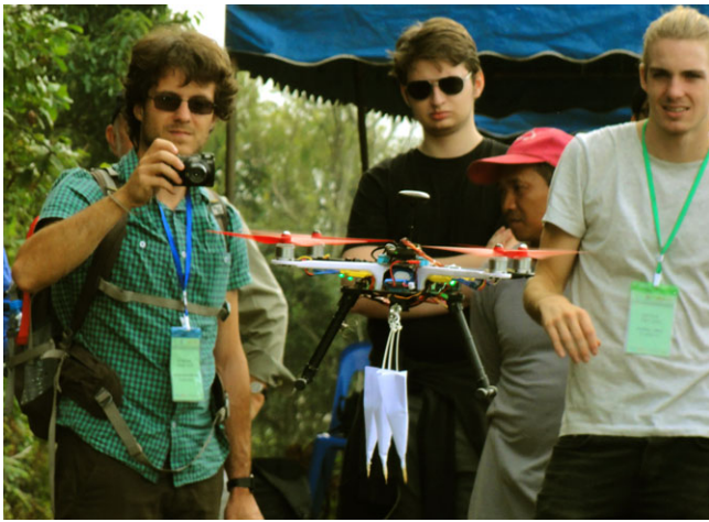
FIGURE 2. Seed bombs can be as simple as paper cones, containing seeds in forest soil, mixed with polymer gel. The drone, pictured here was made by Chiang Mai University Physics Department and releases the bombs using a simple rotating spiral (from the 1st Workshop on Automated Forest Restoration, Chiang Mai University, October 2014).
