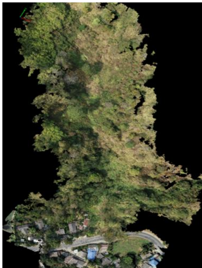
Figure 2: Orthomosaic overview of the sites of pre-planting, using Pix4D mapper demo combine 387 images, taken by DJI Phantom 4 Professional Drone did flight planning at altitude 80 metres above ground
