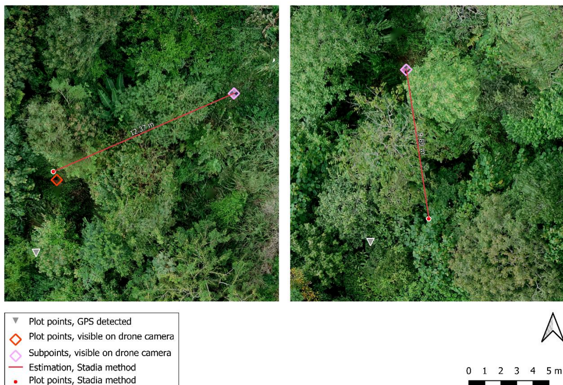
Figure 4.3 Examples of stadia method and comparisons with GPS detected points in orthophoto of BPK site. (Left) Plot point was visible on UAV-derived image (actual plot point; red square) and estimated using stadia method (red point) from visible subpoint (pink square). Two points were closer than the distance between GPS detection (grey triangle) and actual plot point. (Right) ground marker was not visible, and plot point was estimated using stadia method. Results of stadia method at the three sites, where it was necessary, are presented in Appendix C.
