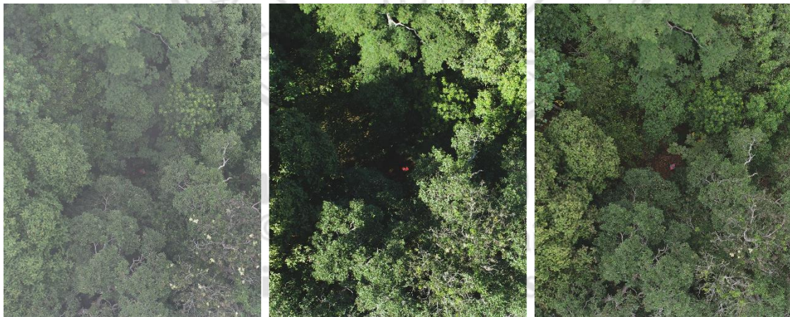
Figure 4.18 Examples of different quality of UAV-derived RGB images from various weather condition in ML site (1,290 m a.s.l.). (Left) cloud interrupted condition, 13:42 PM, 4th September, 2020, (Center) high contrast from strong sunlight, 14:16 PM, 26th October, 2020, (Right) comparatively stable light contrast without obstacles, 11:30 AM, 9th November, 2020.
