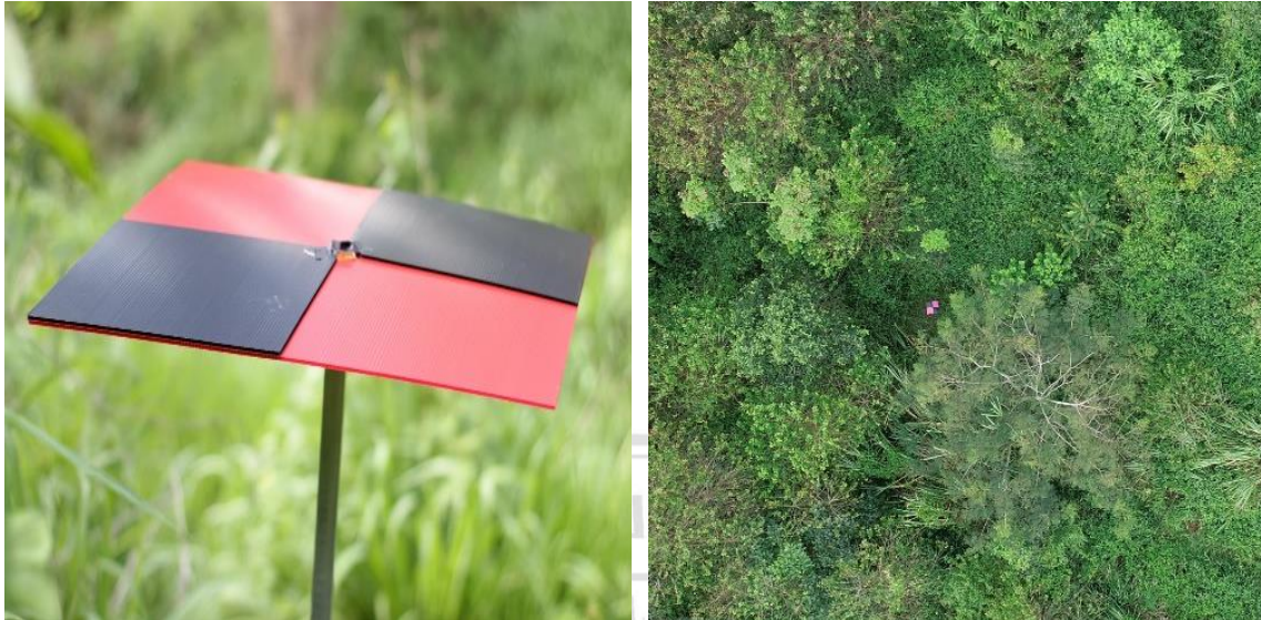
Figure 3.5. (Left) red-black ground marker set at the center of circular plots, (Right) red-black ground marker, detected by UAV image sensing
