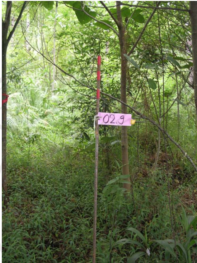
Figure 3.8 the aluminum pole was set on the center of circular sampling units
